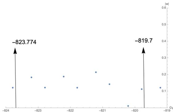
Figure 1: He3 intrinsic spin resonance strength for 10 mm-mrad normalized emittance near the proposed store energy of  $G\gamma = -819.7$ . We also show our results for the  $G\gamma = -823.774$ .
