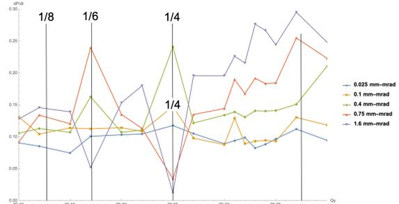
Figure 3: He3 Polarization lifetime at store energy of  $G\gamma = -823.774$ , for various emittances with RMS orbit distortion of 0.5528 mm. The locations of the strong snake resonances are indicated at 1/8, 1/6, 1/4 and 3/8 fractional tunes.
