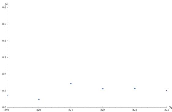
Figure 2: He3 imperfection spin resonance strength for RMS orbit of 0.5528 mm near the proposed store energy of  $G\gamma = -819.7$ .
