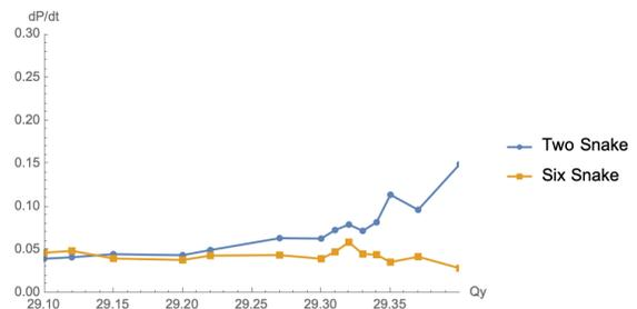
Figure 4: He3 Polarization lifetime at store energy of  $G\gamma = -819.7$ , for 0.75 mm-mrad normalized emittance with RMS orbit distortion of 0.5528 mm.
