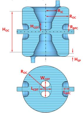
Figure 2: Parametrically deigned HWR.
