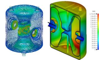
Figure 4: Lorentz force density (left) and the displacement (right) normalized to the stored energy 1 J.
