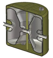
Figure 3: Reinforced design of the cavity and the helium jacket.
