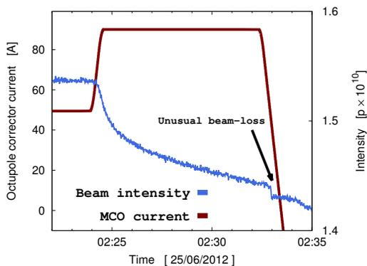
Figure 1: Bunch intensity with increasing and decreasing octupole current.
