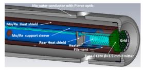
Figure 7: Detailed view of the cathode-grid area.
