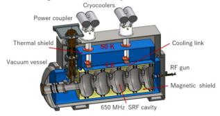
Figure 1: General layout of the 4½-cells cavity SRF linac.
