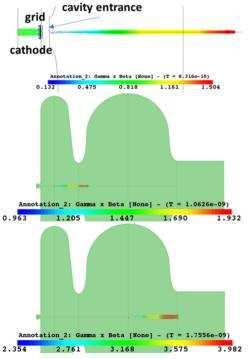
Figure 3: MICHELLE plots of the beam profile.
