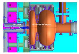
Figure 2: 1½ cells prototype general view.
