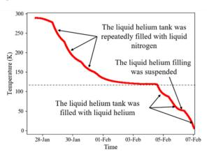
Figure 3: TGU temperature during the cool-down process.
