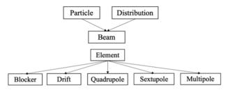
Figure 1: The two main hierarchical class structures in the code: the definition of the beam and the magnetic elements.
