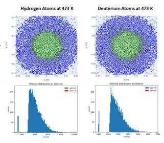
Figure 4: Results of tracking simulations for both hydrogen (left) and deuterium (right) at 200 °C from the source endtube to the detector. Shown in the top are particle coordinates at the detector plane. The green dots are atoms of interest accepted in the detector while in blue are lost atoms, in black are atoms of opposite spin being rejected. The bottom plots are the velocity distributions of the selected atoms accepted in the detector.
