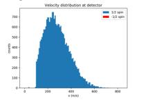
Figure 2: Velocity distribution at the detector for a hydrogen molecular beam following the same set-up and conditions as in [6]. Blue refers to particles with positive spin moment projection and red would be for negative momentum if there were at the detector.
