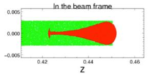
Figure 3: Muons (red) passing through hydrogen gas leave a beam-induced plasma trail (green).
