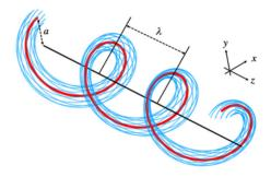
Figure 1: Typical beam paths in a HCC (blue), around a design reference orbit (red).
