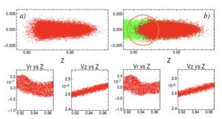
Figure 4: WARP simulations show the plasma lens effect without gas (a) and with gas (b). A red point is an incident particle and a green one is an ionization electron. Only a straight solenoidal magnetic field and RF field are applied, with no dispersion in this simulation. The orange circle shows that the beam is focused by the plasma lens.
