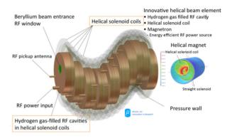
Figure 2: Pictorial drawing of an HCC channel.
