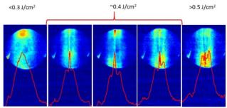
Figure 3: Raw AC images obtained with a single 10 cm thick NaCl slab at a variable input fluence.
