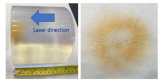
Figure 4: Colour centers formation with micro-filament traces observed after exposing a NaCl slab to CO<sub>2</sub> laser pulses of over 500 mJ/cm<sup>2</sup> fluence.
