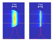
Figure 5: Raw AC images obtained at 450 mJ/cm<sup>2</sup> incident laser peak fluence without post-compression (left) and with a two-element KCl+BaF<sub>2</sub> compressor (right).
