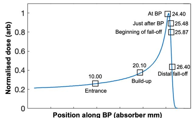
Figure 3: Observed depths along the BP for the different PMMA blocks.
