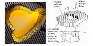
Figure 1: Multi-Leaf Collimator Photograph (left) and schematic depicting an MLC's function (right).
