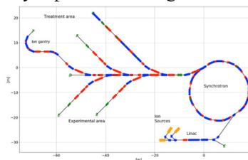
Figure 1: Layout of the synchrotron-based facility.
