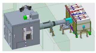
Figure 3: Rendering of NMR's target manipulation system, showing the hot cell joining with the (LTS).
