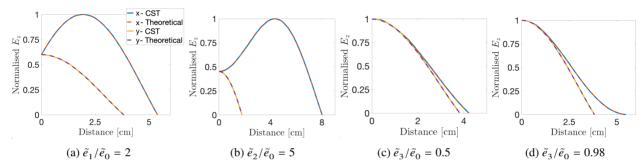
Figure 2: Comparison between simulation (full) to theoretical (dashed)  $E_z$  values normalised to the maximum along the positive, horizontal x (blue and red) and vertical y (yellow and purple) axes.
