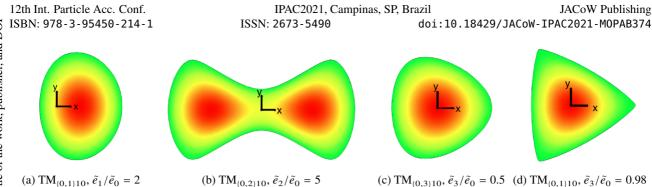
Figure 1: Colour map of the E-fields in four different  $TM_{\{0m\}10}$  cavities (from red as largest magnitude, to green as zero field). The notation  $TM_{\{0m\}10}$  denotes the cavity has been designed to support a mode that contains 0<sup>th</sup> and  $m^{th}$  order multipolar terms and the value of  $\tilde{e}_m/\tilde{e}_0$  is the multipole to monopole ratio of that cavity design. The origin of the [x, y] coordinate axis is where the beam passes through.
