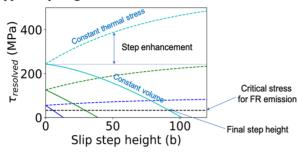
Figure 3: Model predictions for RSS evolution as surface slip step height grows under E-fields of 5 (blue), 15 (green), and 10 (cyan) GV/m and thermal stresses due to 20 °C temperature rise under the conditions described in Table 1.
