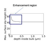
Figure 4: Maximum possible slipped step height at the surface due to emission of dislocation loops from RF sources located at different depths inside the bulk material.
