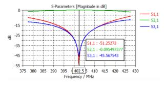
Figure 4: Frequency Domain Response of the DTL Circulator after Tuning (Optimal Tuning Case) [3].
