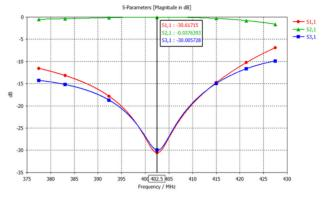
Figure 2: Frequency Domain Response of the DTL Circulator after Tuning.
