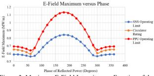
Figure 3: Maximum E-Field Intensity as a Function of the Transmitted Power Phase.
