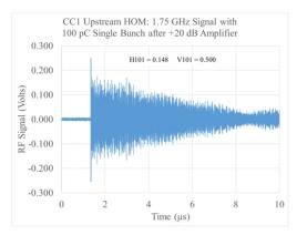
Figure 2: Oscilloscope data from February 2020, showing the 1725 MHz HOM signal level with a single 100 pC bunch and approximately 6 mm of vertical beam displacement.
