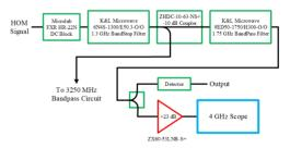
Figure 1: Block diagram of the 1750 MHz section of the Fermilab Prototype. This includes an amplifier (red) added for the February 2020 experiment.
