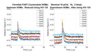
Figure 6: Output of the SLAC chassis with a single bunch of 10 pC and the beam approximately on axis (see text). Both cascaded amplifiers are enabled in all channels.
