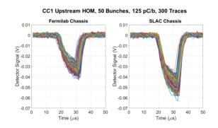
Figure 4: Overlay of 300 traces of CC1 data taken under the same beam conditions with the Fermilab and SLAC prototypes. The electron beam is 50 bunches at about 125 pC/bunch with a spacing of 333 ns.
