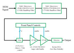
Figure 3: Block diagram of the SLAC prototype channel. There are four channels per chassis
