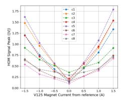
Figure 7: Plot of the SLAC chassis output versus steering magnet current with one amplifier enabled in each channel. The electron beam was 50 bunches at 400 pC/bunch.
