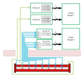
Figure 5: Block diagram of the cryomodule with its connections to the Fermilab and SLAC chassis and Fermilab's ACNET data acquisition system.
