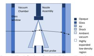
Figure 5: The deflection of a single light ray (Top view).
