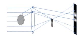
Figure 2: Formation of schlieren image of gas flow.
