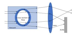
Figure 6: Deflection of light in the schlieren setup by the cross section of the flow.
