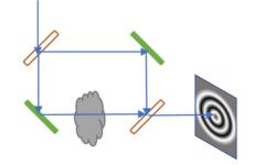
Figure 3: Formation of interference image of gas flow.
