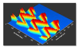
Figure 1: BSM measurement successfully proving the beam energy modulation around 160 MeV, programmed to optimize the multi-turn injection process into the PSB.
