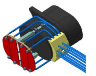
Figure 4: PSB H<sup>0</sup>-H<sup>-</sup> beam current monitor installed after the H<sup>-</sup> striping foil units: four plates integrate the signal from non stripped ions before they are absorbed by the dump.
