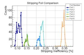
Figure 6: Stripping inefficiency as measured by the H<sup>0</sup>-H<sup>-</sup> monitor in the PSB Ring 3 during dedicated studies with different foil types (preliminary results).
