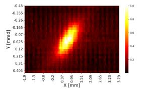
Figure 2: LINAC4 beam phase space horizontal distribution, as measured by the new laser emittance meter, in the L4 -PSB transfer line.
