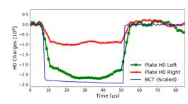
Figure 5: Measurement of the only partially non stripped particles  $(H^0)$  as measured by the dedicated monitor in front of the dump.
