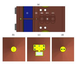
Figure 2: PAH and apertures. (a) Overview of apertures in PAH. (i) XBPM1 electrodes (in blue). (ii) BL1 (beamdefining aperture for XBPM2). (iii) BL2. (iv) BL3. (v) BL4. (b) Enlarged image of BL2 slit defining horizontal relative beam size monitor. (c) Enlarged image of BL3 apertures defining absolute beam size monitor. (d) Enlarged image of BL4 apertures defining vertical relative beam size monitor.
