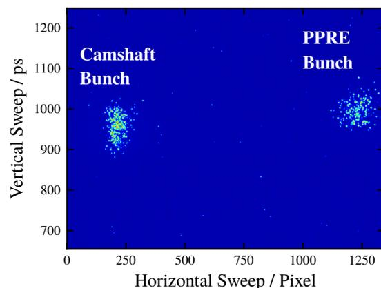
Figure 1: Single-shot single-turn streak camera measurement from the camshaft and the PPRE bunch at the new diagnostics beamline.
