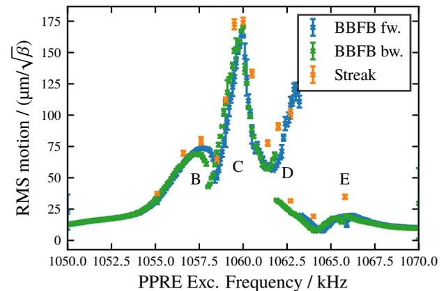
Figure 7: Horizontal PPRE bunch motion measured with the streak camera and the BBFB system (for two scanning directions) as a function of the PPRE excitation frequency, normalized by the horizontal  $\beta$ -function at respective source points.
