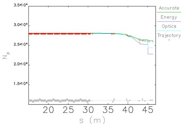
Figure 4: Beam losses in the electron injection channel.
