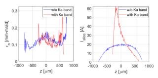
Figure 4: Electron beam slice analysis in terms of emittance (left) and peak current (right) at the photo-injector exit spaces with (red line) and without (blue line) the Ka-band linearizer.
