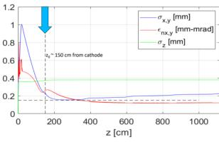
Figure 3: Evolution of the electron beam transverse normalized emittance (red line), transverse spot size (blue line) and bunch length (green line) without linearizer until the photo-injector exit.
