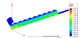
Figure 2: 3D model of one-eighth of half a SW structure simulated with the HFSS software. The surface electric field is shown for a 125 MV/m on-axis accelerating gradient.
