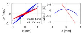
Figure 5: Transverse and longitudinal phase space at the photo-injector exit spaces with (red line) and without (blue line) the Ka-band linearizer.
