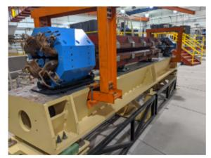
Figure 1: Photograph of one half of the double achromat cell used in the 2018 upgrade of the south arc of the CESR ring.
