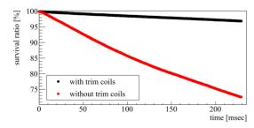
Figure 4: Beam survival ratio as a function of circulating time with and without the trim coils.
