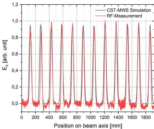
Figure 5: Simulated and measured electric field distribution on the beam axis of the FoS-Alvarez (RF-measurement: uncoppered cavity).
