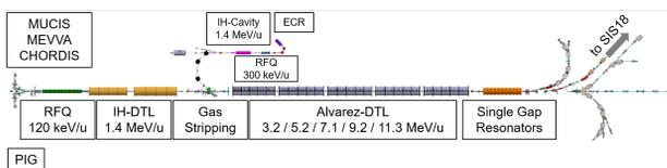
Figure 1: Schematic overview of the new GSI UNILAC.
