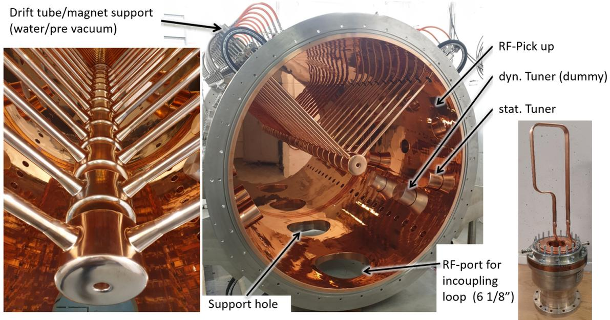
Figure 3: The copper plated FoS-Alvarez cavity section with a length of 1.9 m and 11 drift tubes. The drift tubes are installed at the top of the tank, but other combinations are possible. The bottom houses RF coupling, a support hole. Two vacuum pumps are installed from the side at the FoS cavity. (right) The new inductive incoupling loop for a 6 1/8" rigid line.
