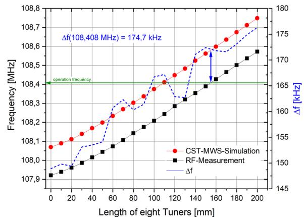
Figure 4: Simulated and measured frequency of the FoS-Alvarez depending on the position of the plungers (RF-measurement: uncoppered cavity). (blue) Frequency difference between simulation and measurements.
