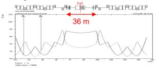
Figure 3: Layout with betatron functions for the RR-10 straight section, adapted for foil injection. A  $\sim$ 36 m segment between focusing quads is reserved for injection kickers, injection bump magnets and stripping foil.
