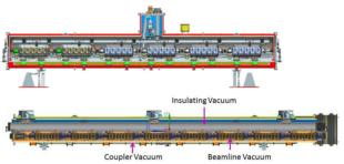
Figure 2: Cross-sections of 650 MHz (above) and 1300 MHz cryomodules, showing cavities and other components [1, 5].
