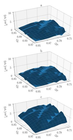
Figure 5: Dynamic aperture of AGS sorted by rigidity: a) helions at  $|G\gamma| = 7.5$ ,  $B\rho = 6.968$  Tm; b) protons  $at|G\gamma| = 4.5$ , helions  $B\rho = 7.203$  Tm; c)  $|G\gamma| = 10.5$ ,  $B\rho = 10.780$  Tm.
