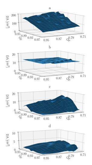
Figure 4: Comparison of DA for helions at  $|G\gamma| = 7.5$  with: a) snakes off, no limiting aperture; b) snakes off with limiting aperture; c) snakes on, no limiting aperture; d) snakes on, with limiting aperture.
