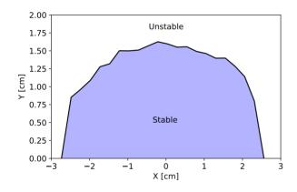
Figure 3: Example dynamic aperture in the AGS with  $v_x = 8.77$  and  $v_y = 8.88$ .
