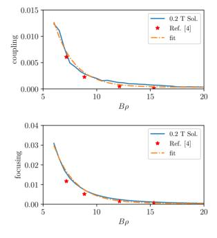
Figure 1: Coupling and focusing from the AGS cold snake as a function of  $B\rho$  and comparison to an exponential function.
