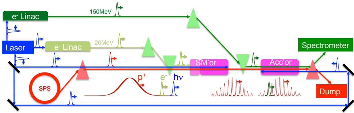
Figure 1: Schematic set-up for Run 2 experiments showing the plasmas (pink colors) for SM (SM'or) with the density step, and for acceleration (Acc'or), as well as the two linacs and beamlines (green colors) for the seeding electron bunch (20 MeV) and the bunch for acceleration (150 MeV). The various bunches (protons in red) and laser pulses (blue color) are also schematically shown. Not to scale.
