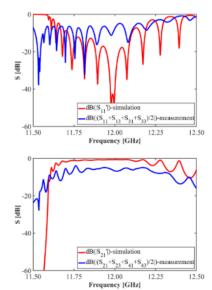
Figure 10: Comparison between measured and simulated S-parameters.
