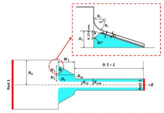
Figure 6: Geometry of a chamfered dielectric matching section with a vacuum microgap, and a DLA structure.
