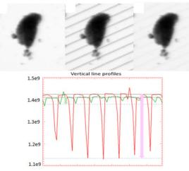
Figure 2: Top: Raster scans in I08 with no disturbance (left), injection magnets (middle), and both PMs (right). Bottom: Vertical slices through the middle (red) and right (green) plots.
