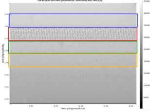
Figure 5: Intensity variation with no disturbance (blue), injection magnets (red), injection magnets and horizontal PM (green), injection magnets with both PMs (yellow).
