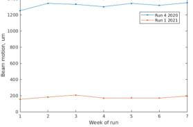
Figure 7: Peak-to-peak stored beam motion monitored over 7 weeks. Blue shows a run without PMs operating, red shows a run with PMs operating.
