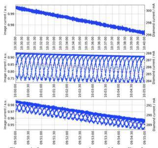
Figure 4: Image current at mirror with no disturbance (top), injection magnets only (middle) and injection magnets with both PMs (bottom).
