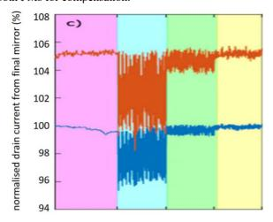
Figure 3: Intensity for hard (red, offset by +5%) and soft (blue) x-rays with no disturbance (left, pink), injection magnets only (centre-left, cyan), injection and horizontal PM (centre-right, green) and injection and both PMs (right, vellow).
