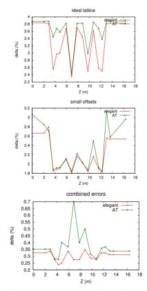
Figure 6: Momentum aperture in AT and elegant, for three lattices with varying error models.
