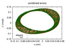
Figure 1: Comparison of turn-by-turn particle trace in AT and elegant, in phase space, for several error types combined.
