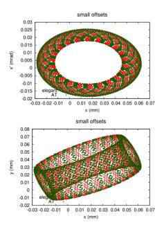
Figure 4: Comparison of turn-by-turn particle trace in AT and elegant, for small offset errors, in phase space (top) and coordinate space (bottom).
