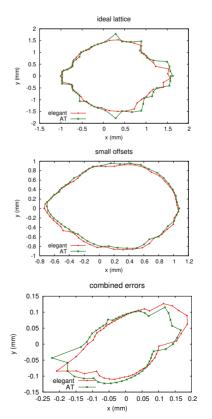
Figure 5: Dynamic aperture in AT and elegant, for three lattices with varying error models.
