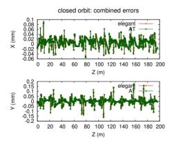
Figure 3: Comparison of closed orbit in AT and elegant, for several error types combined.
