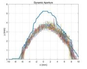
Figure 6: Dynamic aperture at injection point (100 seeds).
