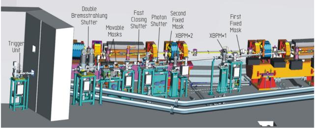
Figure 5: Layout of FE for FAXTOR.
