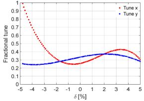
Figure 4: Transverse tune shifts with momentum, tracked for 1024 turns.
