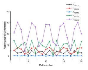
Figure 1: Changes of the third-order resonance driving terms with the cell number.
