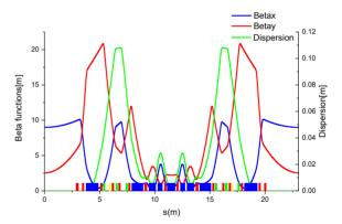
Figure 2: Linear optical functions and magnet layout of the selected lattice.
