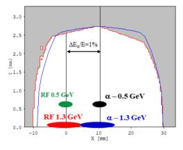
Figure 2: Expected images of RF and  $\alpha$ -buckets to be simultaneously stored at KARA during low- $\alpha$  operation where the first term of momentum compaction factor is  $\alpha_1$ =+1·10<sup>-4</sup>. Bunches at 0.5 and 1.3 GeV are split in the vertical plane for clarity. Dispersion D $\approx$ -1m at observation point. It was assumed that momentum offset between RF and  $\alpha$ -buckets is  $\approx$ 1%.
