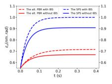
Figure 1: Emittance (hor.) evolution on the injection plateau of the SPS (blue) and the alternative PBR design (red).
