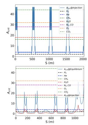
Figure 2: Critical mass for the alternative PBR (top) and one sextant of the SPS (bottom) in comparison to the thresholds for various molecules.
