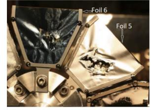
Figure 1: The stripping foils 5 and 6 after they were removed from BtA line. They are still attached to their holders and still on the foil wheel. Foil 6 has a Carbon coating on top of the Aluminum which makes it black.
