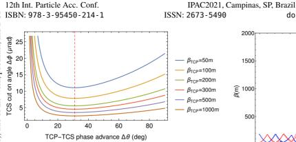
Figure 1: Example of cuts from the TCS on the scattering angle of particles exiting the TCP, as a function of the TCP-TCS phase advance  $\Delta\theta$ , for several different values of  $\beta_{\text{TCP}}$ . Typical numerical value for the LHC proton operation have been used:  $n_1 = 6$ ,  $n_2 = 7$ ,  $\epsilon_n = 3.5 \,\mu\text{m}$ ,  $\gamma_{\text{beam}} = 7461$ . The dashed vertical line shows the optimum phase advance  $\Delta\theta_{\text{opt}}$  from Eq. (2).
