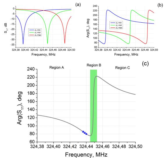
Figure 3: (a) Frequency dependencies of reflected from the cavity signal  $S_{11}$  for plunger positions with minimal, middle, and maximal penetration depth  $\Delta L$ ; (b) the same for  $S_{11}$  phase; (c) 3 points positions in Algorithm B.
