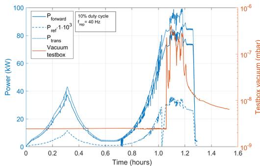
Figure 4: Intermediate result of first condition series with 1<sup>st</sup> pair reaching about 90 kW forward power at 10 % duty cycle with 40 Hz repetition rate displaying the three power signals and testbox vacuum with time.
