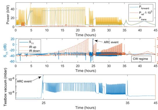
Figure 7: Part of the conditioning series of the 2<sup>nd</sup> coupler pair displaying peak power,  $S_{11}$  parameter, ceramic window temperature and testbox vacuum with time.
