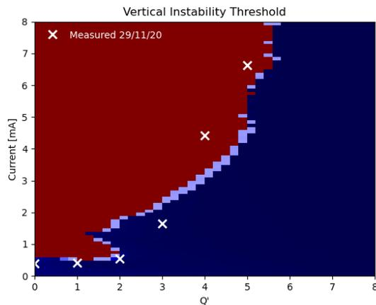
Figure 6: Vertical instability threshold as a function of chromaticity. The white crosses are measurements, the shaded regions show the area of stability (blue) or instability (red).
