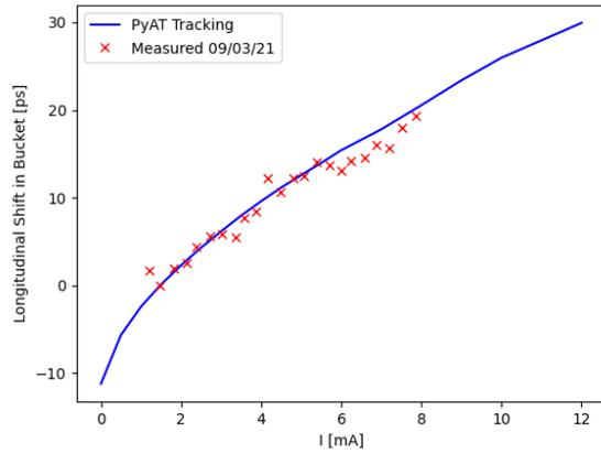
Figure 3: Longitudinal shift of the bunch versus current, compared to simulations. The noise of the data will be reduced in the future with new settings for the streak camera.
