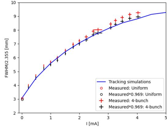
Figure 2: The measured bunch length versus single bunch current compared with simulations. No difference was measured between gaps open or gaps closed.
