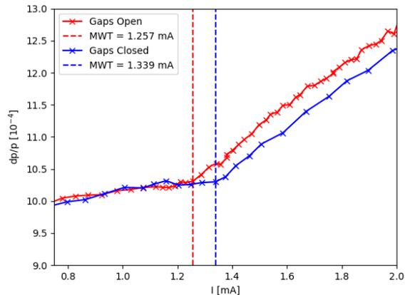
Figure 4: Measured MWTs for IVU open and closed. The simulated threshold is not shown but was calculated as 3.5 mA. Gaps open threshold is lower due to the large taper angle of the IVU tanks.
