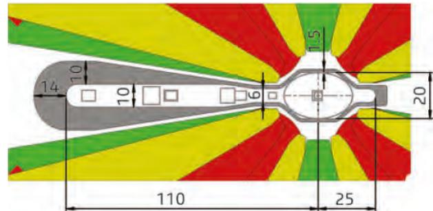
Figure 1: The vacuum chamber profile. The beam passes through the chamber on the right hand side, while the ante chamber on the left is for the synchrotron radiation. For the impedance modelling, only the profile close to the beam is considered.
