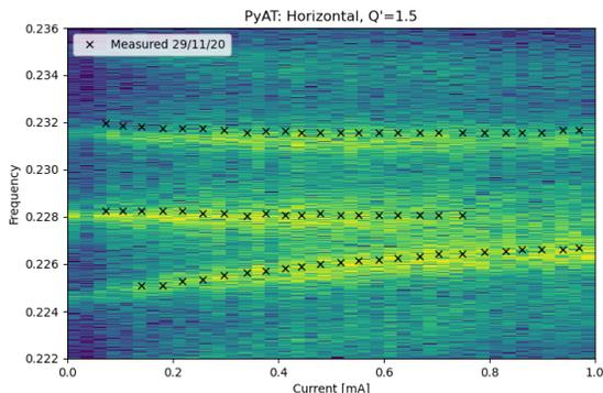
Figure 5: Horizontal mode shift at  $Q'=1.5$ . The black crosses are peaks coming from the measured spectrum, whereas the colored background is the simulated spectrum.
