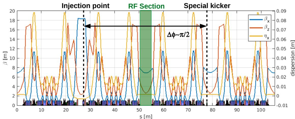
Figure 2: Proposed layout for the ESRF-EBS lattice.
