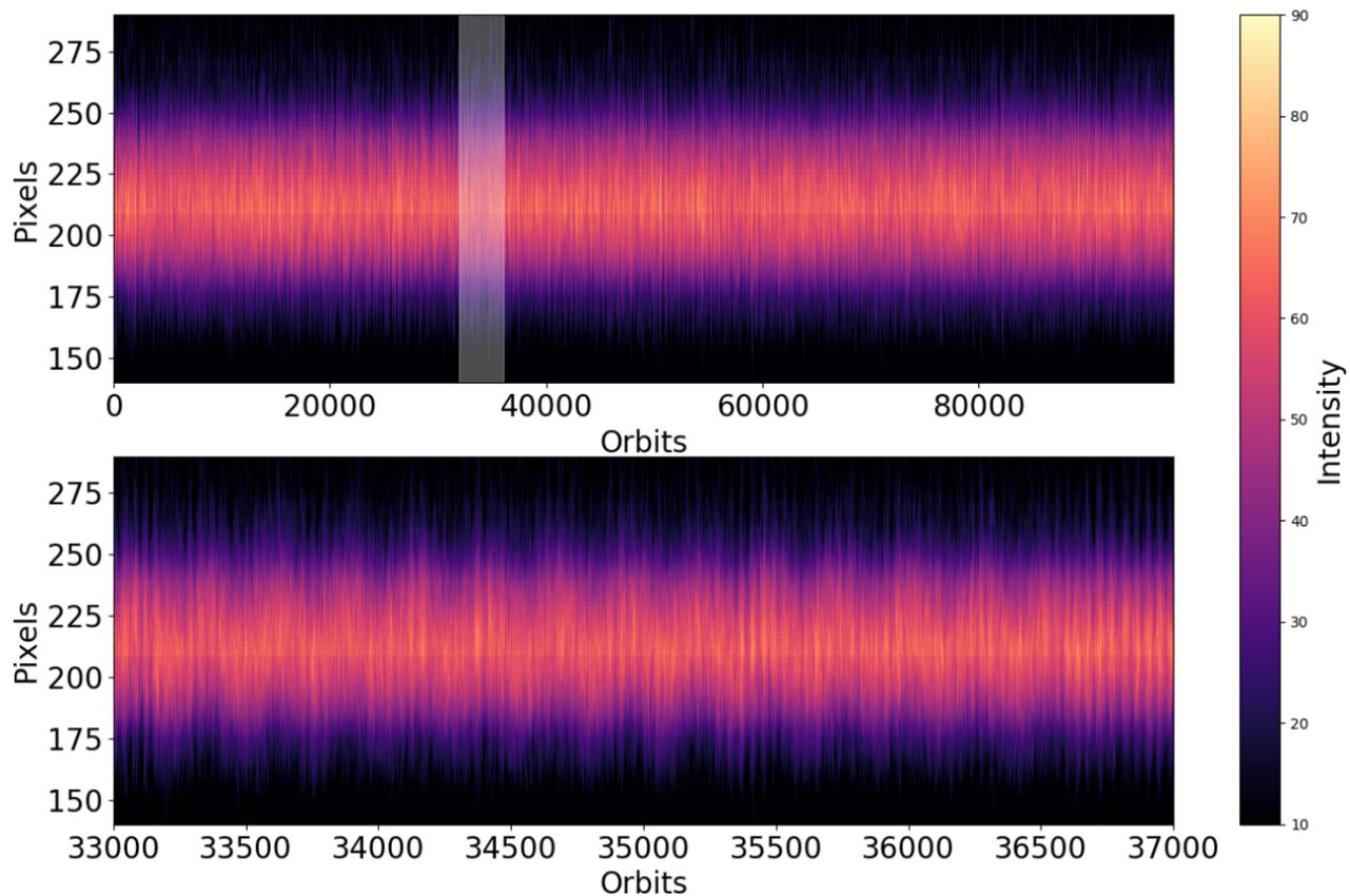
Figure 9: Raw measurement data of the incoherent synchrotron radiation recorded with KALYPSO over multiple turns. The acquisition rate of KALYPSO was set to 2.7 Mfps. Each vertical line corresponds to a single-shot and turn-by-turn measurement. The synchrotron oscillation of the electron bunch is visible on the bottom plot. The full data-set consists of  $10^5$  turns.
