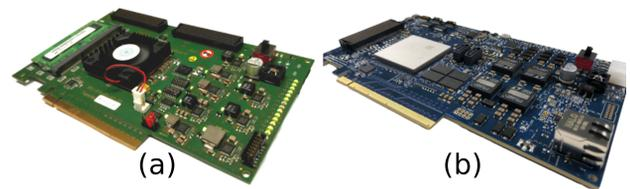
Figure 5: Back-end data acquisition systems developed at KIT, (a) Hi-Flex v1 based on Virtex 7 FPGA with FMC connector, (b) Hi-Flex v2 based on Zynq Ultrascale+ with FMC+ connector.
