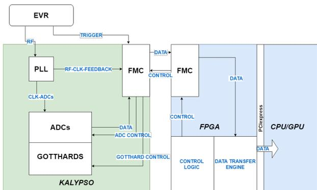
Figure 6: Data and control flow implementation in KALYPSO.
