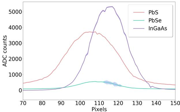
Figure 3: Laser beam profile measured with the infrared sensors.
