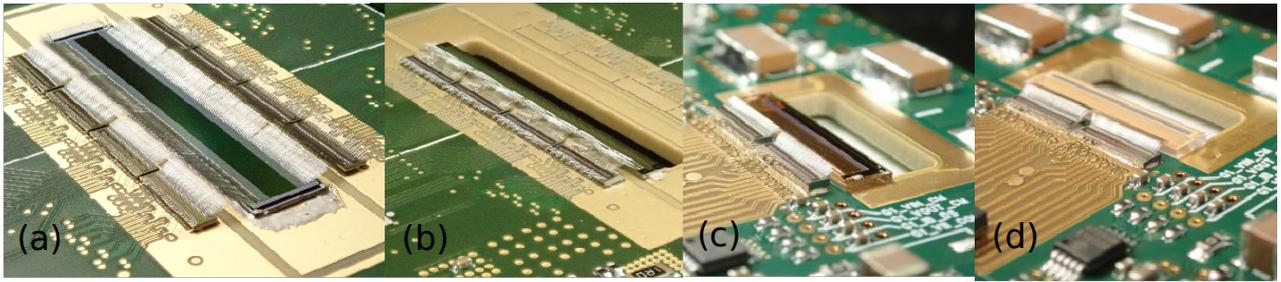
Figure 2: KALYPSO-board mounted with different micro-strip sensors. (a) Si, (b) InGaAs, (c) PbS, (d) PbSe.
