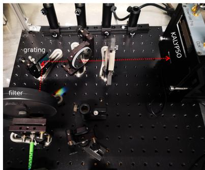
Figure 7: EOSD optical and data acquisition setup at KARA for the measurement of longitudinal bunch profile of the electron beam.
