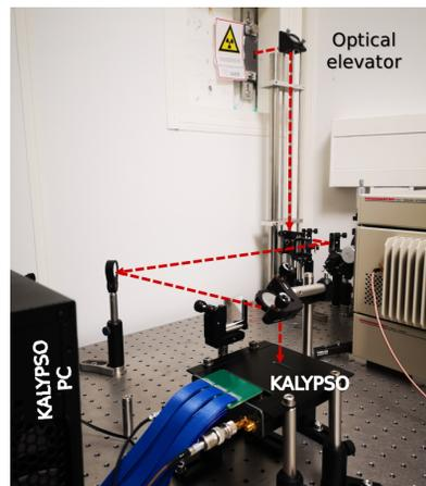
Figure 8: Optical and data acquisition setup for the horizontal bunch measurement for energy spread studies at KARA.
