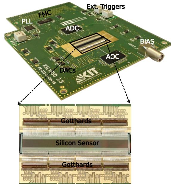
Figure 1: A fully mounted KALYPSO-board based on silicon with 1024 pixels sensitive to the visible light spectrum.
