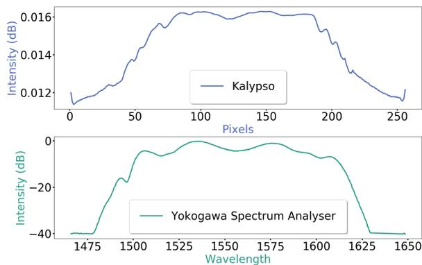
Figure 10: Spectral measurements of a 1 560 nm commercial laser as measured by KALYPSO at a frame rate of 2.7 MHz compared to the measurement with a commercial spectrometer.
