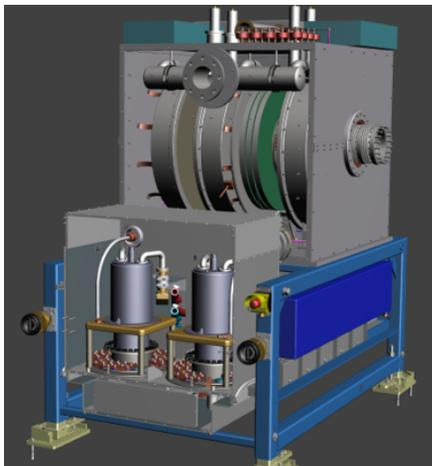
Figure 8: Visualization of a possible broadband cavity and amplifier system from the „Research and Development-study for magnetic alloy broadband cavities“ (Aurion Anlagentechnik GmbH)
