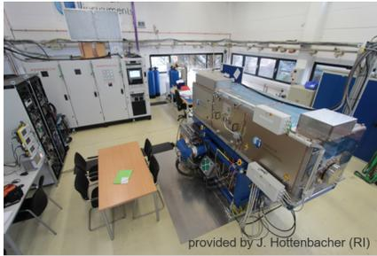
Figure 2: Test stand for factory acceptance tests of the cavity and amplifiers at RI (courtesy of RI Research Instruments GmbH).
