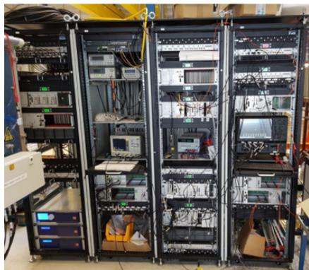
Figure 6: Installation of the LLRF racks in the test stand of the AC first of series RF station at GSI.
