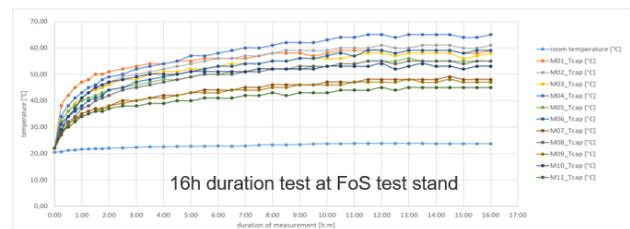
Figure 4: Temperature on the power supply unit anode modules stabilize at  $\sim 65^\circ\text{C}$  during a 16 h duration test on the cavity.
