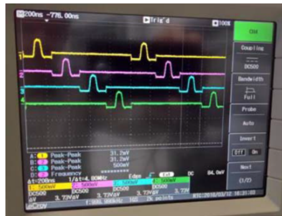
Figure 9: Measurement of demultiplexed bunch signals of an emulated chain of 4 bunches.
