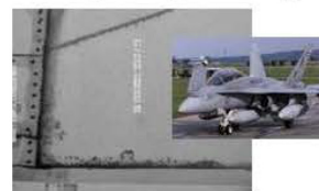
Neutron image of H2O penetration in F18 honeycomb
