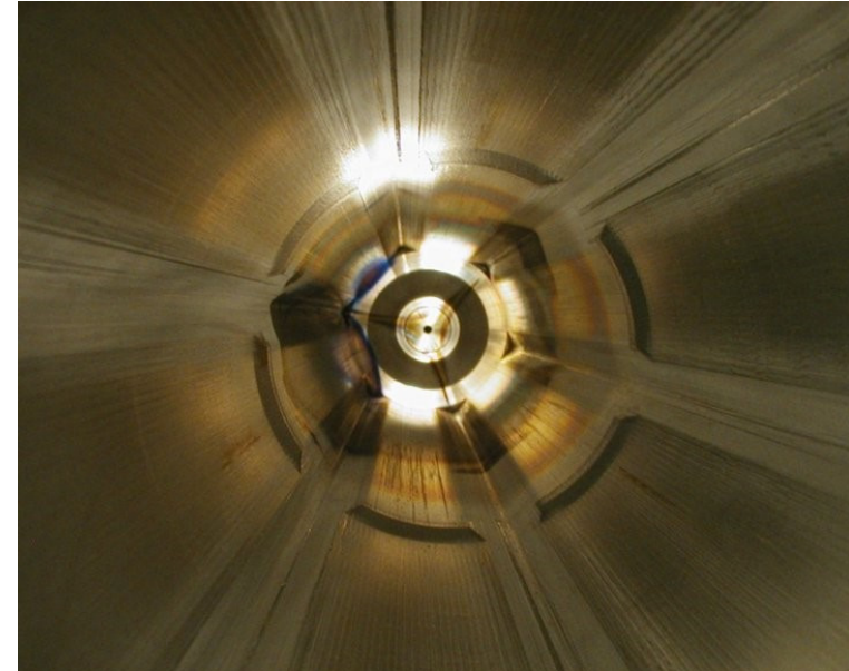
View into the plasma chamber of the VENUS ECR Ion Source
