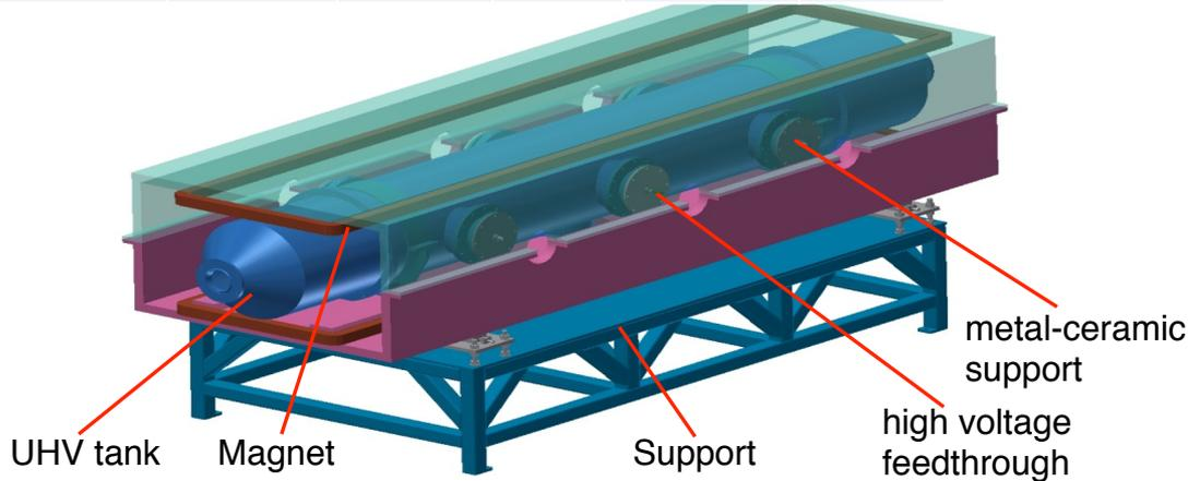
structure drawing of Electrostatic-Magnetic Deflector
