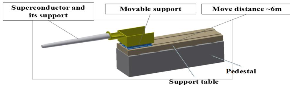
Schematic of support system of superconducting magnets
