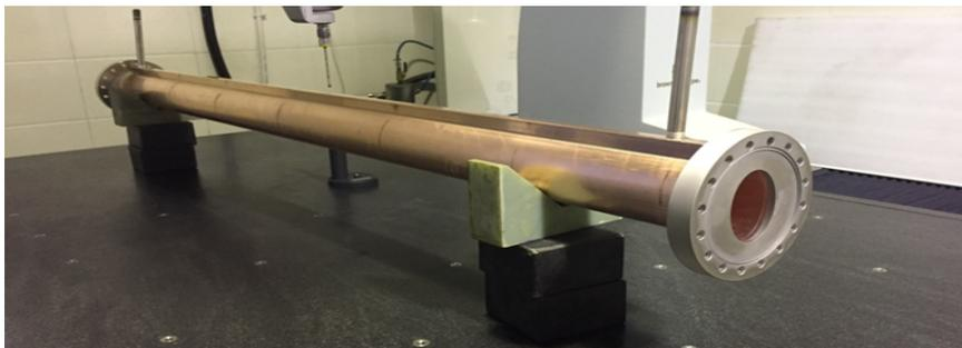
1.5m long copper vacuum chamber prototype
