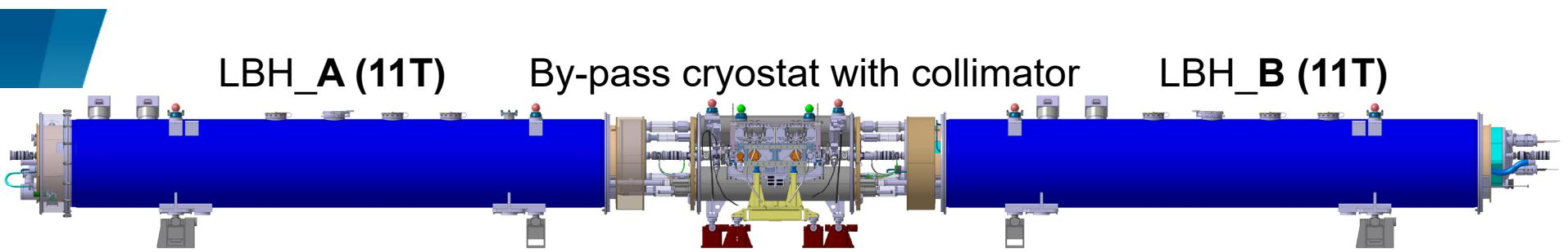
**Complete 11.2 T cryo-assembly replacing a 15 m 8.3 T LHC dipole in 2020**
