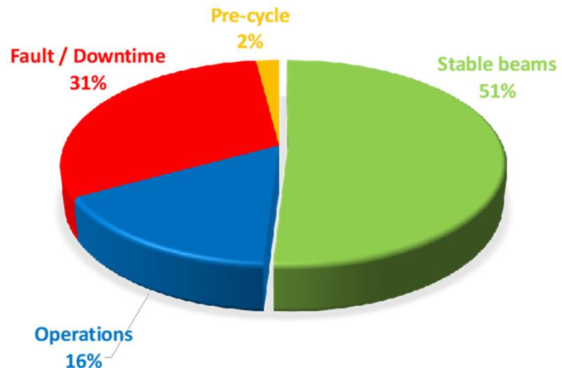
Typical figure for Run 2. this means 70% machine (including injectors) availability and about 60% efficiency!
