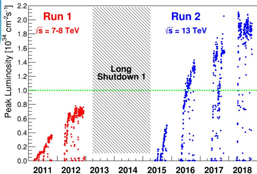
Limited by the heat deposition in the IT Quadrupole in Nb-Ti: forecast 1.7- 2  $L_0$  ( $L_0 = 10^{34} \text{ cm}^{-2}\text{s}^{-1}$ , LHC nominal design lumi)
