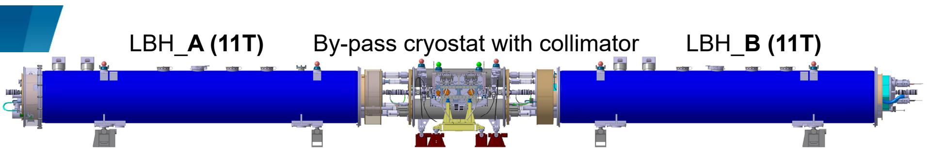
**Complete 11.2 T cryo-assembly replacing a 15 m 8.3 T LHC dipole in 2020**
