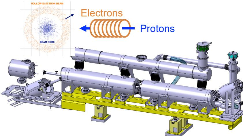
*It would allow controlling actively the halo, through a hollow electron beam (overlapped over three meters to the proton/ion beams) that selectively excites halo particles.*
