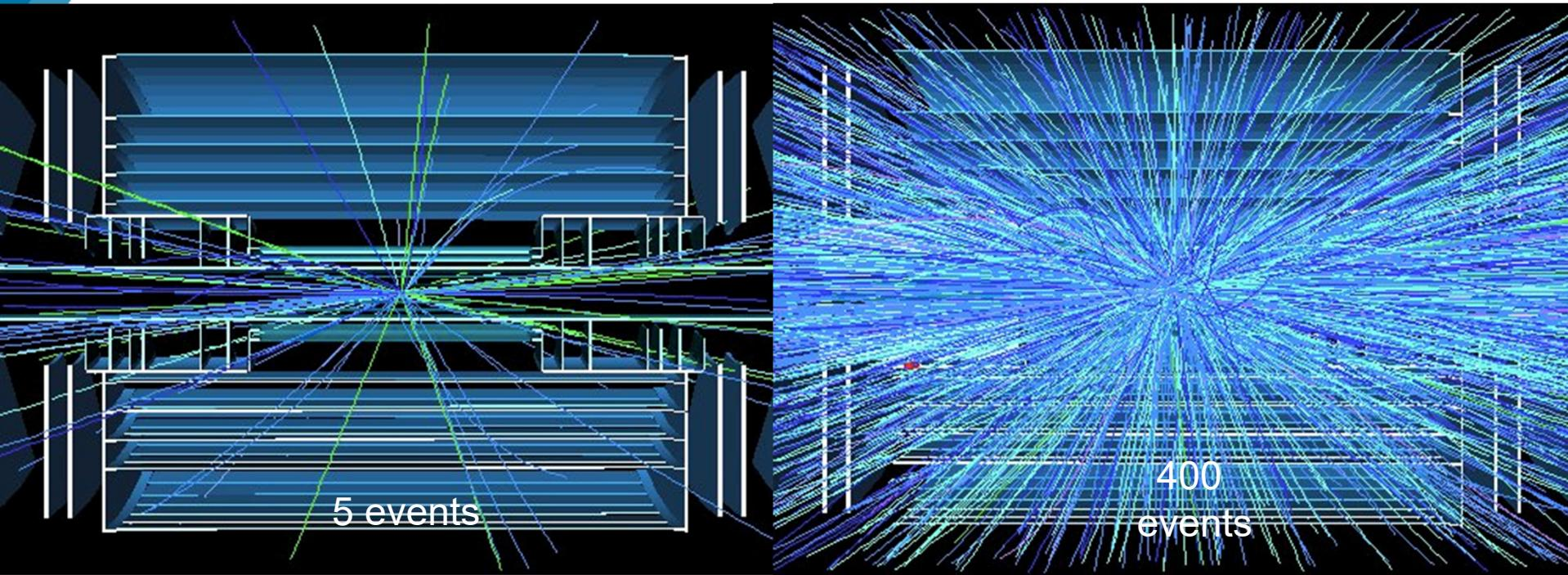
Pushing at the maximum the parameters of HL-LHC we would start the fill at  $L = 17 \times 10^{34}$  with **400 events/crossing**.
