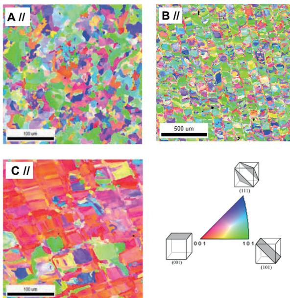
Figure 3: EBSD images for AM 316L samples, side parallel to the build plate, from different manufacturers (A, B and C) and standard stereographic triangle.
