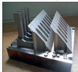
Figure 1: Example of additive manufacturing build plate.
